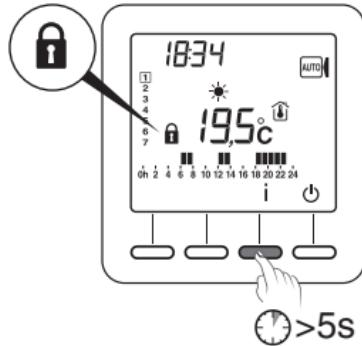
To enable the beeps again, press the i button for 5 seconds.
