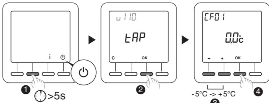
**The thermostat must be in shutdown mode.**
