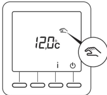
During the external override, if the symbol
