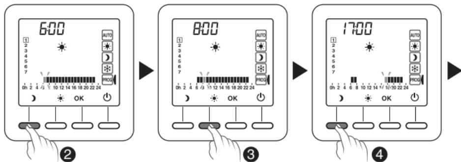
Programming can be made by steps of 1 hour or 1/2 hour (configuration menu CF11).
